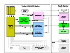
Fig. 5: HiSCORE-9 DAQ2-system as used for this analysis, with DRS4-Evaluation Board and White-Rabbit timing system. Left: Station setup (with DRS4-EB, WR-SPEC and Rasp-MiniPC). Right: Schematics of the setup in Station and Center for DAQ-2 (DAQ-1 in grey) [6].
