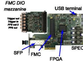
Fig. 2: Example of a WR-Node: The SPEC card, the WR-node used for this work. The precision time, kept on the Spartan-6 FPGA is synchronized through the fiber cable to the central WR-switch. With Mezzanine Digital I/O card. Right: Scheme of modified WR-firmware for time-stamping, clock and triggering [4].
