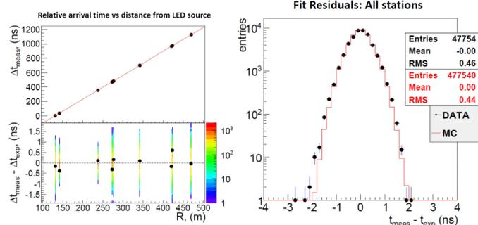
Fig. 8: LED Calibration. Left: Upper panel: station relative arrival times  $\Delta t_{meas}$  as function of distance  $R$  from the LED light source. Red line gives  $t_r = R/c$ . Lower panel: fit residual distributions per station. Black dots show an example of a single triggered event. Right: Distribution of fit residuals for LED events (all nine stations superimposed). Black dots: data; Red line: simulated events. [6]
