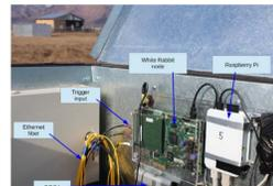
Fig. 4: The complex HiSCORE WR field-setup, as operated in 2012/13 to evaluate time-synchronization and nsec-trigger time-stamping by monitoring WR-nodes. Right: HiSCORE prototype station with DAQ and WR components.
