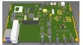
Fig. 3: A next generation Node: WR-ZEN - based on Xilinx-Zynq (2xARM9) + FMC [3].
