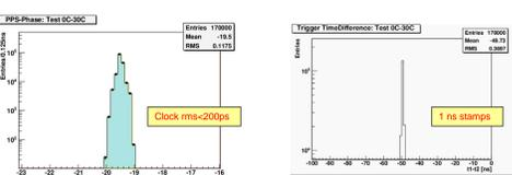
Fig. 7: Sub-nsec precision timing in climate chamber tests. Left: Distribution of time difference between PPS clock-pulses from two WR-nodes (SPEC1/2), synchronized by a WRS, for a 48-hour run:  $\sigma=0.12$ ns. SPEC2 card and the 500m fiber-coil were subjected to temperature ramps between 0° and 30°C. For details see [4]. Right: Same run, comparing the digital trigger timestamps (1ns resolution) generated on the WR-SPECs:  $\sigma=0.37$ ns (time-offsets  $\neq 0$  are due to cabling).
