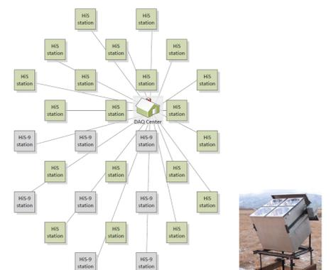
Fig. 6: HiSCORE-28 array layout: 28 stations at 100m spacing forming a super-cell structure, total area = 450x600m<sup>2</sup> (HiS-9 stations are indicated). Right: Optical station with four 8" PMTs, inclined 25° southwards.
