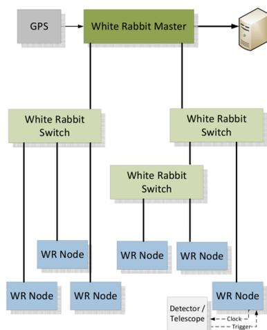
Fig. 1: The White Rabbit network: made up of WR-switches (WRS), Grand Master and normal WRS, and of WR-nodes. The WR-nodes deliver clock-signals to, and/or extract time-stamp signals from the associated detectors (or telescopes), as symbolized for the lower-right WR-node.
