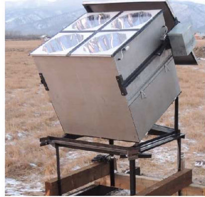
Figure 6: A HiSCORE optical station, with four 8" PMTs and Winston Cones, inclined by 25^\circ southwards.
