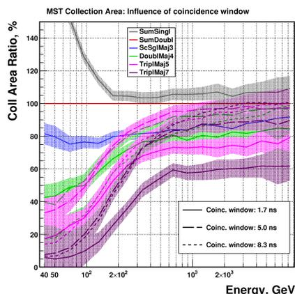
Figure 7: Relative MST collection area as function of coincidence window: 1.7, 5.0, 8.3ns (NSB/AP as in fig.5). At high energy, larger windows are favored.
