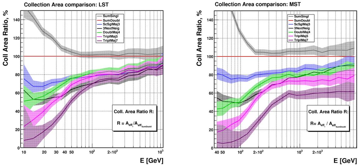
Figure 6: Trigger collection area for LST and MST from fig.5, normalized to Sumtrigger 'SumDoubl'.
