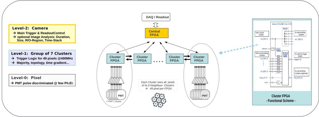
Figure 2: Block scheme of the FPGA-based Camera Trigger. Each *Cluster-FPGA* operates on 49 pixels/PMTs (7 direct and 6x7 neighbouring cluster pixels). *Central FPGA* at camera level: allows for optional Level-2 trigger / image classification. *Right insert*: Functional scheme for each Cluster-FPGA: input (7+42 pixel), digital delay lines, trigger factory, 7-pixel fanout to neighbouring cluster and trigger output (3 bits).
