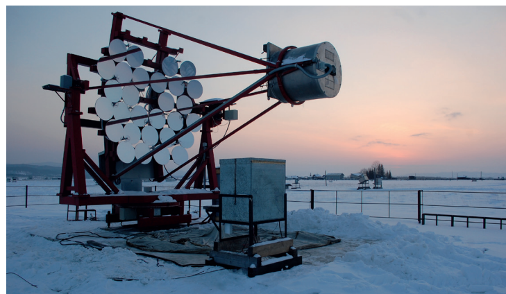
IACT telescope of the TAIGA project, where WR hardware is tested in field conditions in conjunction with an array of Cherenkov light detectors (photo credit: DESY/Ralf Wischnewski).
