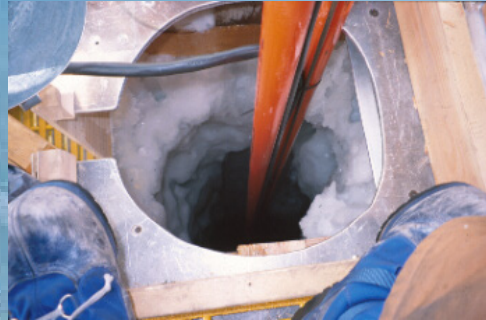
Hot water drilling
