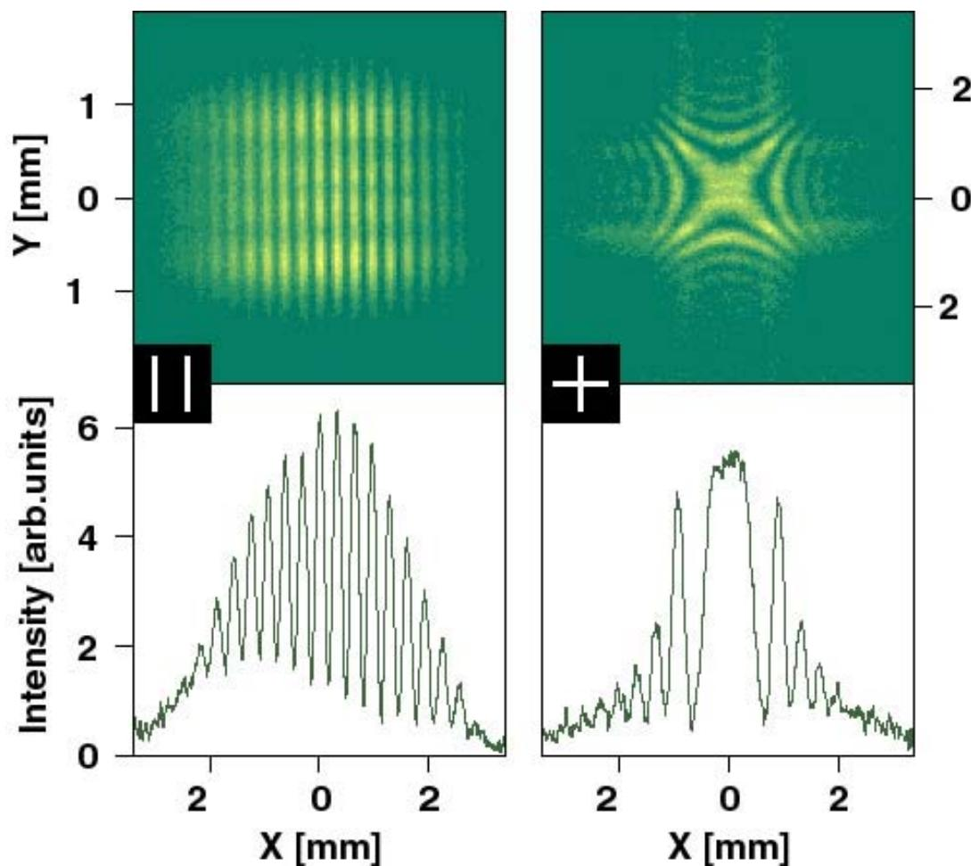
Diffraction of 95 nm FEL radiation from a pair of parallel slits, each 2mm long and 200  $\mu\text{m}$  wide at a distance of 1 mm, and crossed slits, 100  $\mu\text{m}$  wide and 4 mm long. The diffraction patterns were observed by a CCD camera on a Ce:YAG crystal 3 m behind the slits. Slit distance from the FEL  $\sim$ 12 m.
