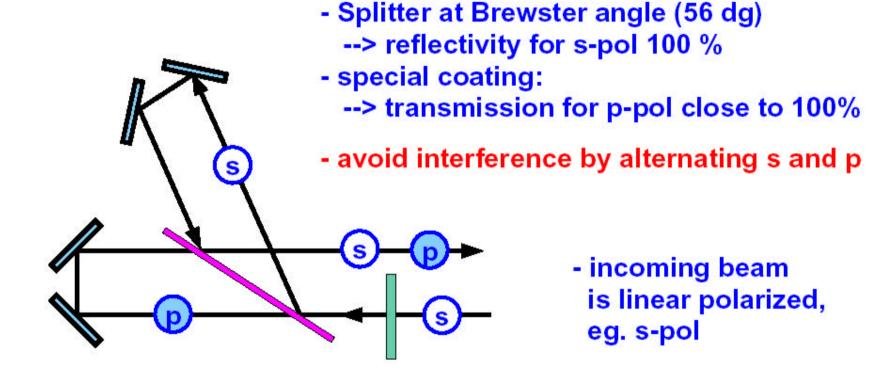
half-wave plate to turn polarisation by 45 dg
