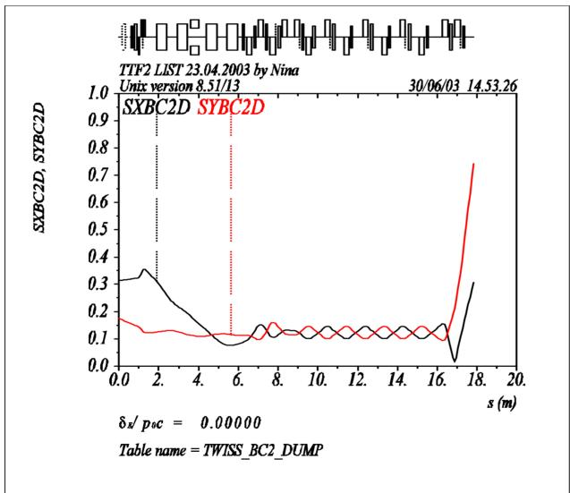
Beam Size in the Bunch Compressor and Diagnostics section with commissioning optics
