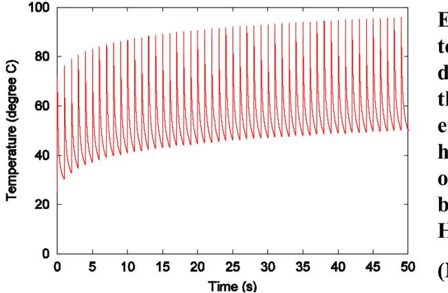
Example of the temperature development in the center of the exit window; high current optics, 125 bunches, 8nC, 1 Hz
