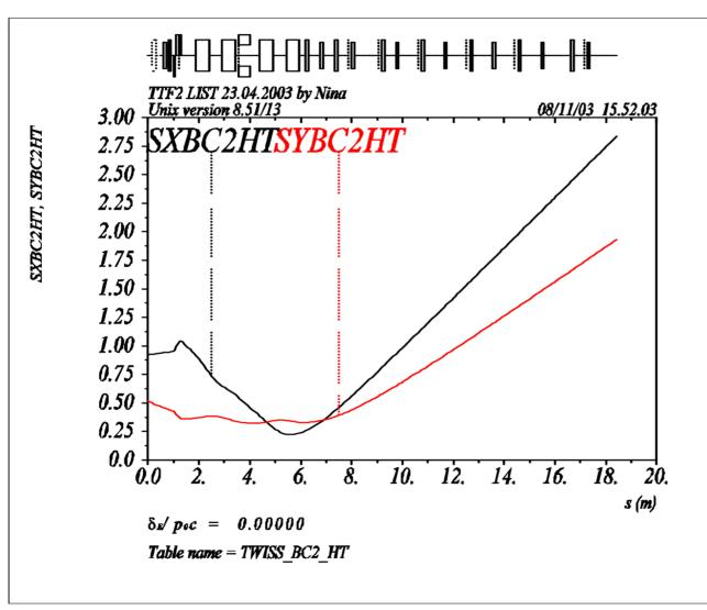
Beam Size in the Bunch Compressor and Diagnostics section with high current optics,
