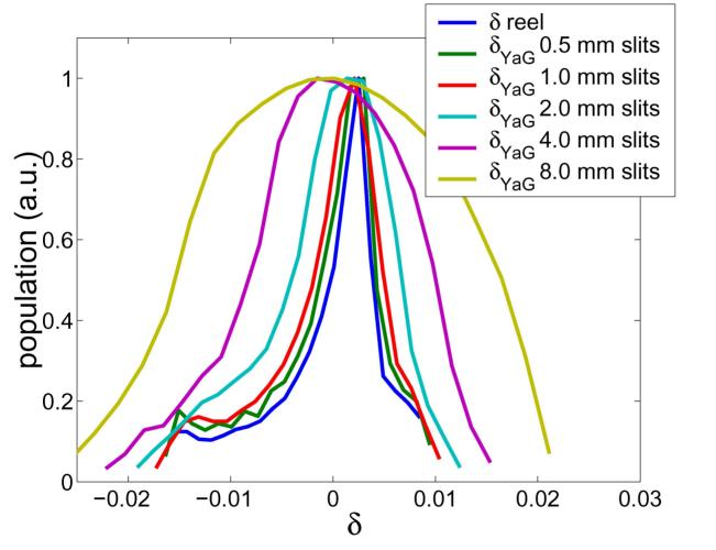
Measured energy profile as function of the slit width
