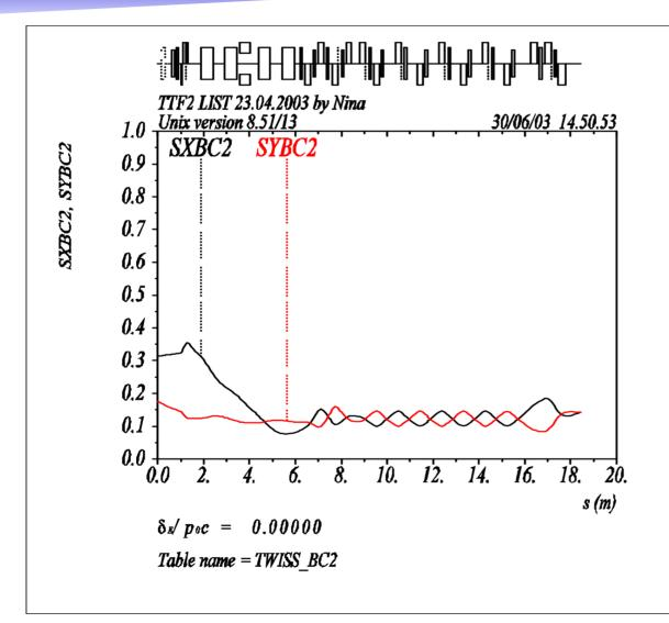
**Beam Size in** the Bunch Compressor and **Diagnostics** section with nominal optics  $\epsilon = 1.10^{-6} \text{ m}$ (N. Golubeva)
