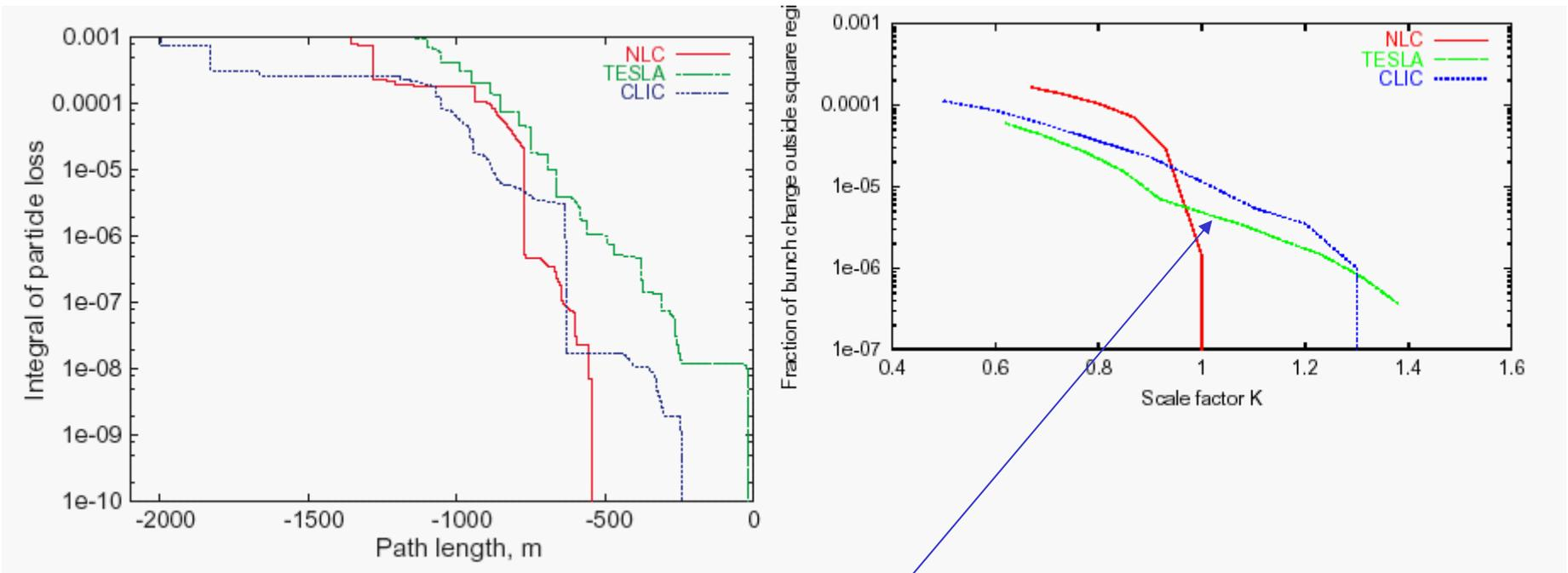
Bad performance of TESLA system *not* due to scattering, but appears to be optics! (confirmed by results of G. Blair)
