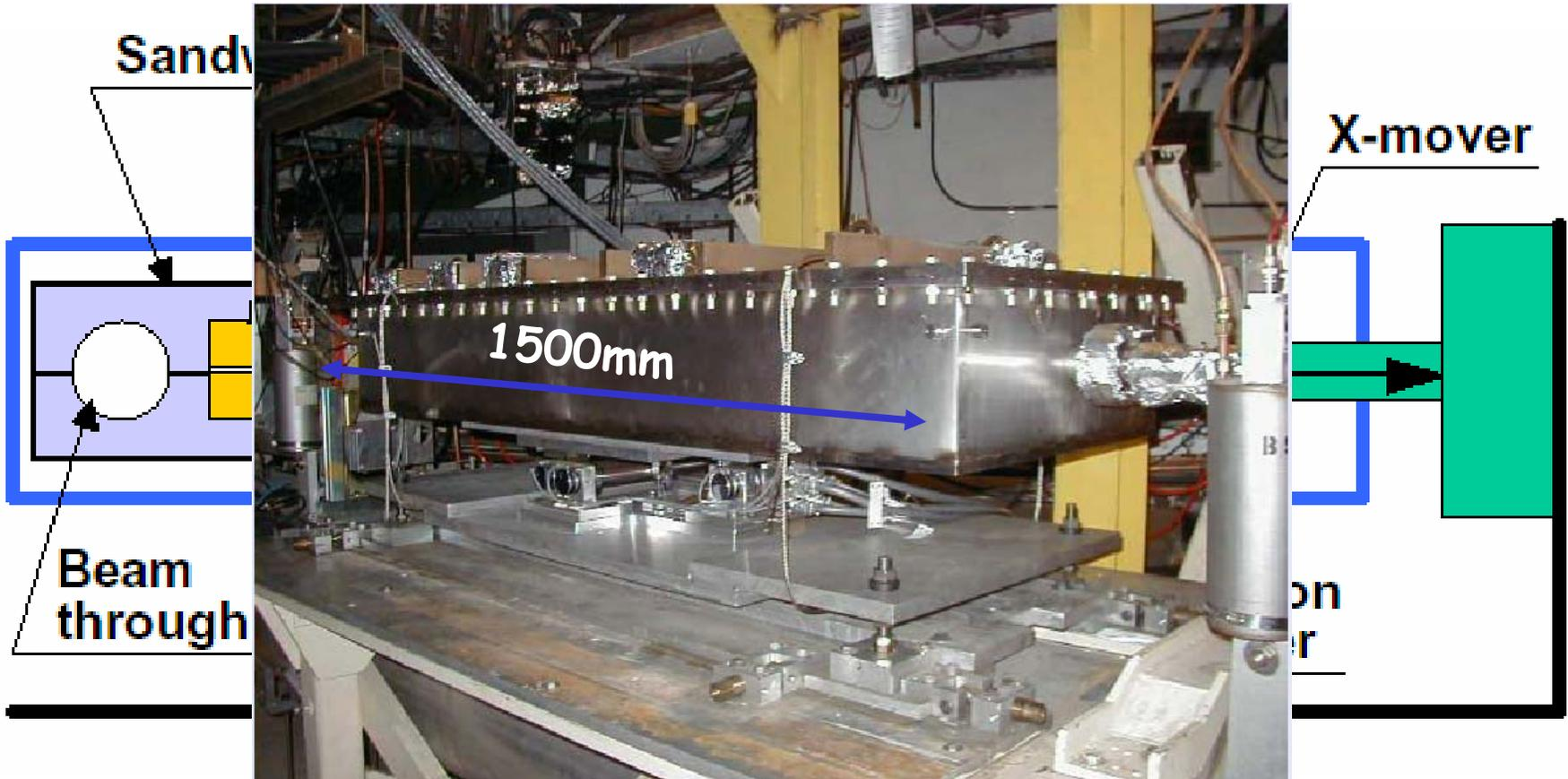
Magnet mover, y range =  $\pm 1.4\text{mm}$ , precision =  $1\mu\text{m}$
