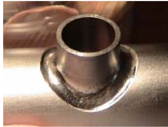
Final, acceptable weld for mounting HOM Coupler
