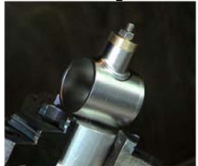
Sample welding to determine weld parameters
