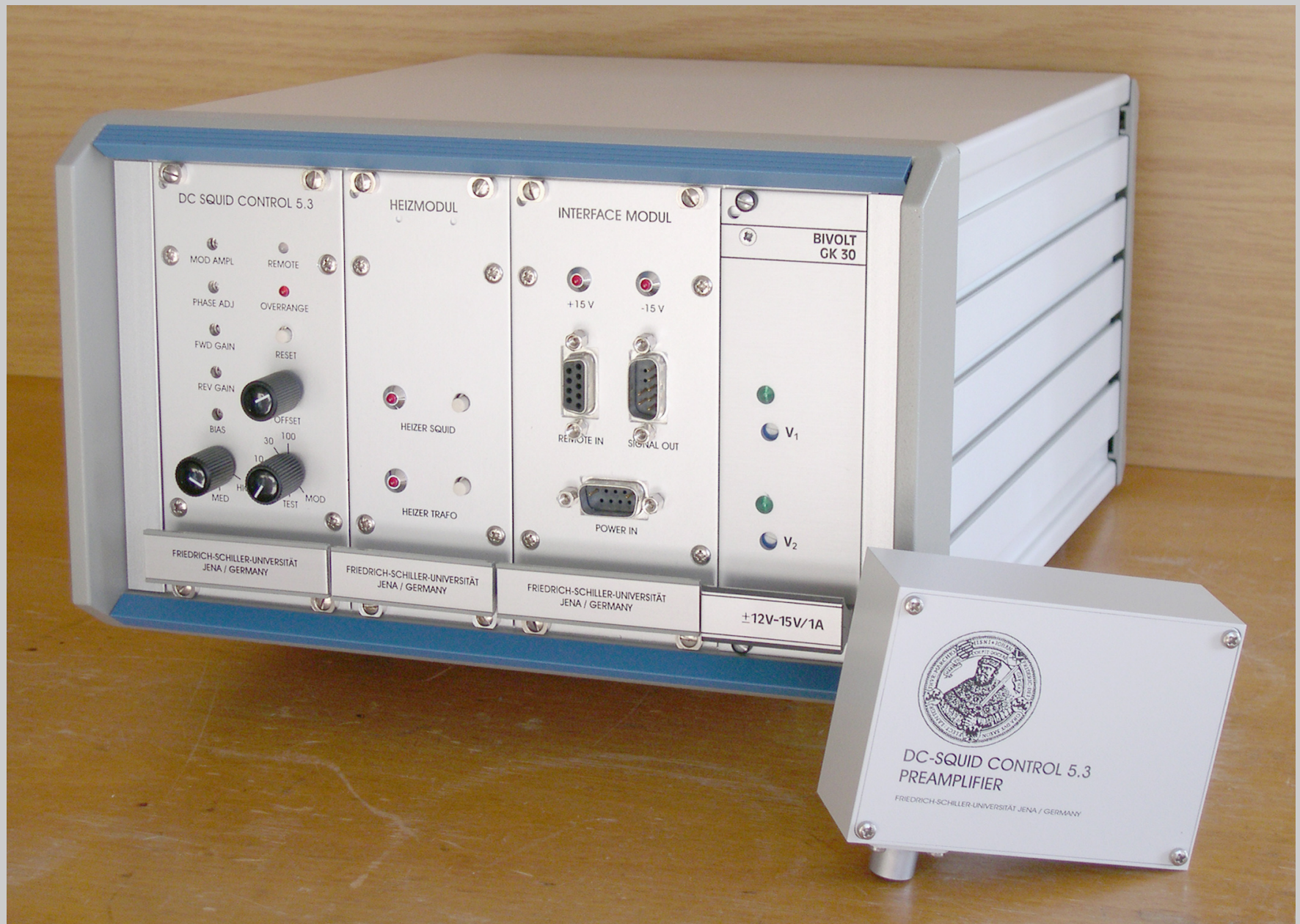
SQUID electronics, custom made for DESY (FSU Jena)
