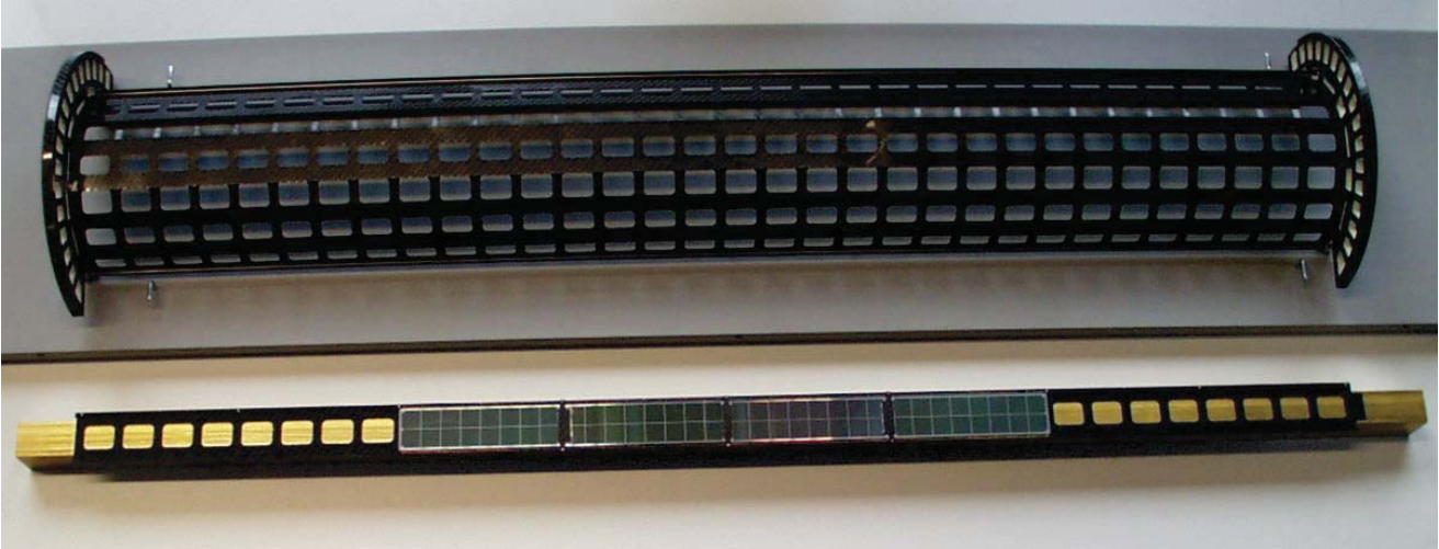
Ultra-leight weight carbon fibre frame and airex end flange with pipes for CO2 cooling.
