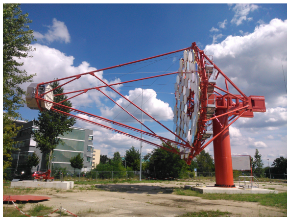
Figure 4: Prototype of the MST located in Adlershof (Berlin). Some of the facets are real, but most of them are dummy mirrors and the camera is a concrete box of approximately the same weight as the real one. This prototype's only purpose was to study the mechanical properties of the instrument.
