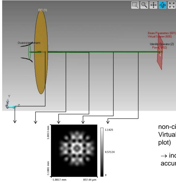
Axicon: Cone shaped optical device used to create quasi-Bessel beams (diffraction free high intensity region)
