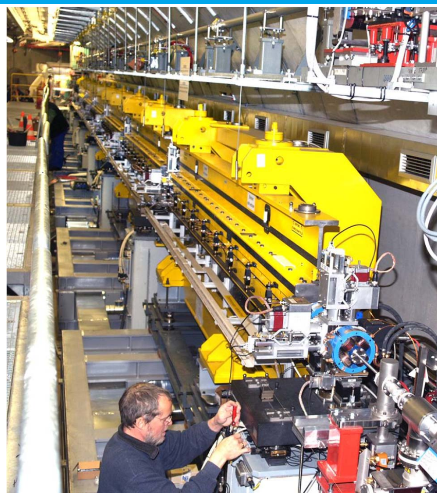
6 undulators (4.5 m long) at FLASH
