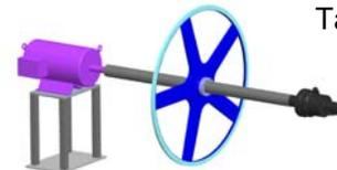
Target wheel (rotating to distribute heat load)
