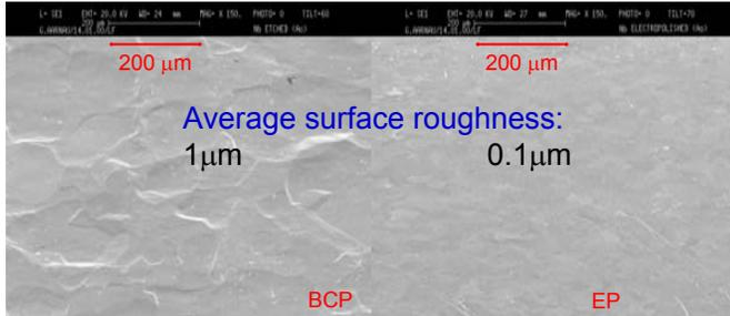
etching - “buffered chemical polish”    electro-polishing
