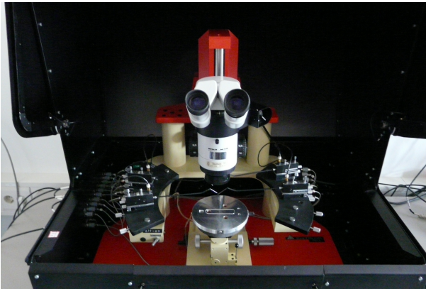
Figure 7: Probe Station, used to connect sensor pads with needles.
