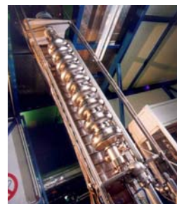
Accelerator module with superconducting niobium cavities 25 MV/m routinely Length: 12 m Weight: about 10 tons!
