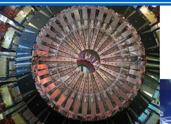
view of CMS HCAL endcap some Cathode Strip Chambers (CSC) can be seen through the central hole
