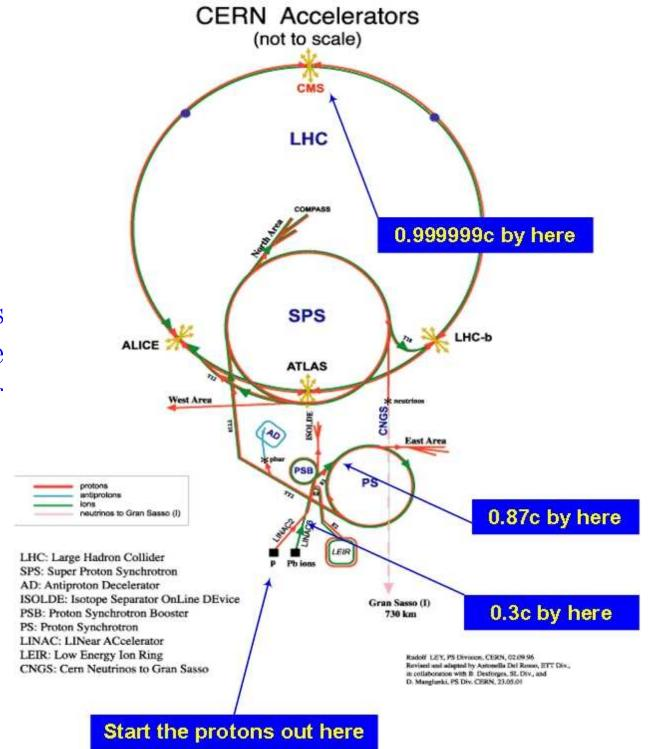
LHC receives its beams from the CERN accelerator complex
