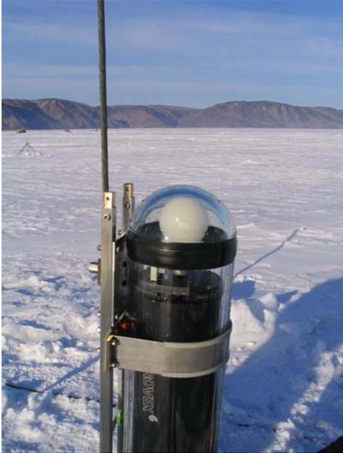
Figure 2: The NT200+ external Laser before deployment in 2005. The white sphere inside the transparent pressure glass cylinder is the isotropizing ball.
