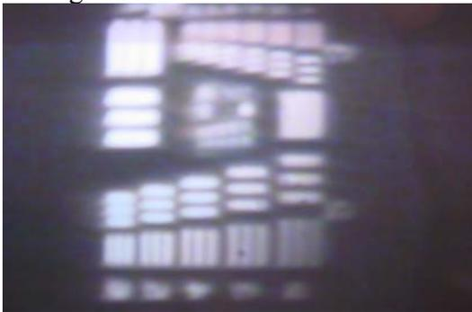
Fig.17: *The picture to estimate the resolution of the setup recorded by a CCD camera*
