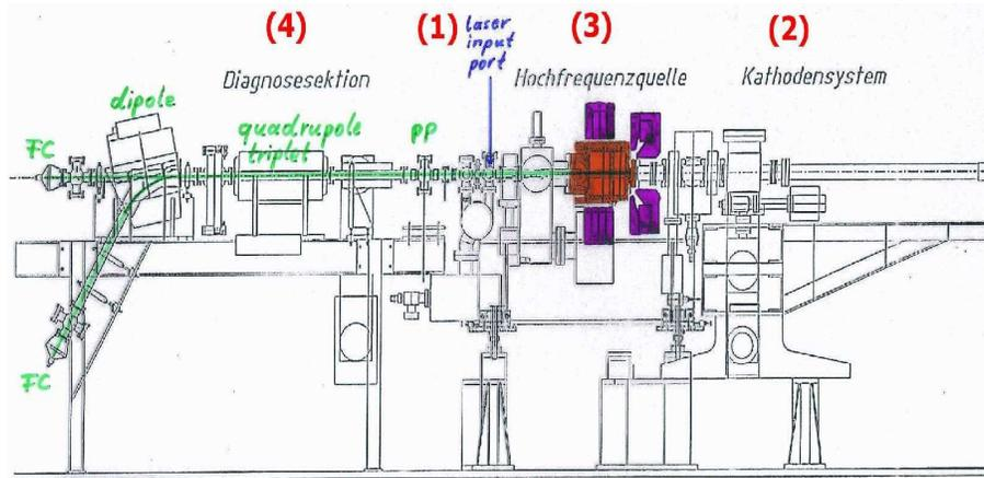
Fig. 1: PITZ setup[?]: (1) Laser input port; (2) Cathode system; (3) RF source and solenoid magnets; (4) Diagnostic section; PP - pepper pot; FC - Faraday cup
