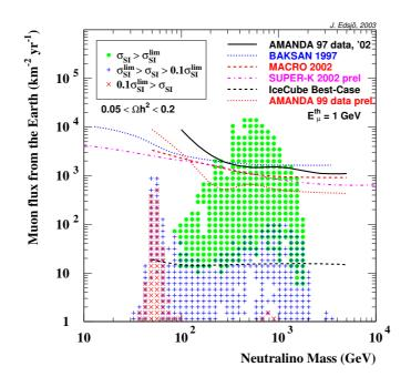
Figure 1: Experimental bounds on the muon flux from the center of the Earth. Additionally shown are muon flux predictions from neutralino dark matter annihilation in the center of the Earth. The filled circles represents models excluded by current direct searches. Crosses represent models which could be excluded by direct searches ten times as sensitive as the present ones. Details concerning the predictions as well as references to other experiments can be found in [3].
