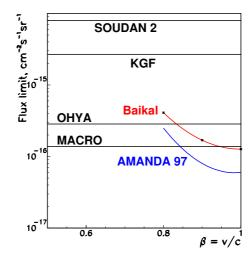
Figure 2: Experimental limits on the flux of relativistic magnetic monopoles as a function of velocity  $\beta = v/c$ . References to other experiments can be found in [4].
