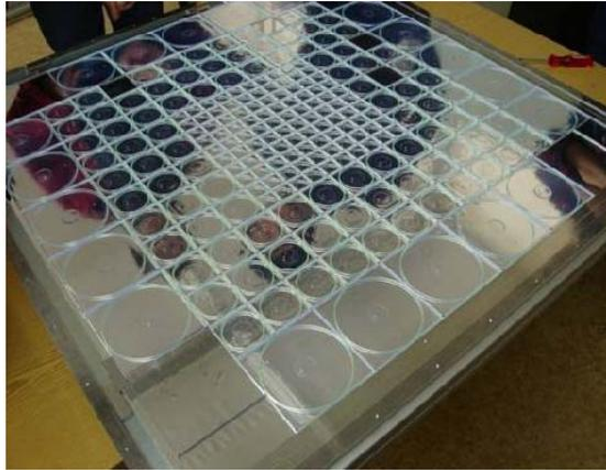
Figure 5: Scintillator HCAL: Photograph of one detector plane
