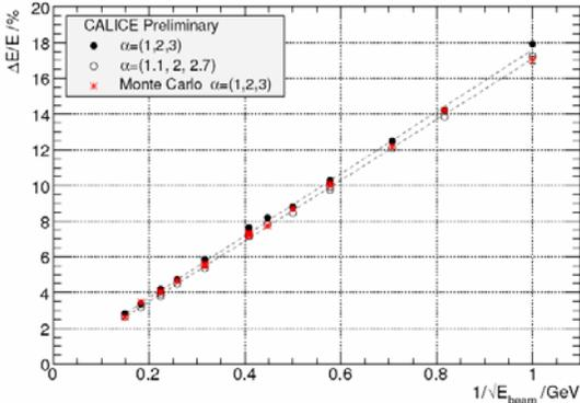
**Figure 2: Silicon ECAL: Energy resolution versus  $1/\sqrt{E_{\text{beam}}}$**
