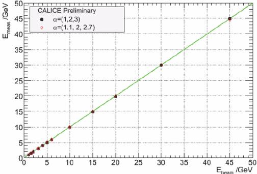
**Figure 1: Silicon ECAL: Reconstructed energy versus beam energy**
