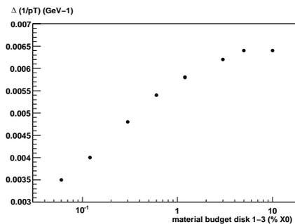
Figure 2: The transverse momentum resolution for 1 GeV tracks in the LDC forward tracker versus material budget in the innermost disks.
