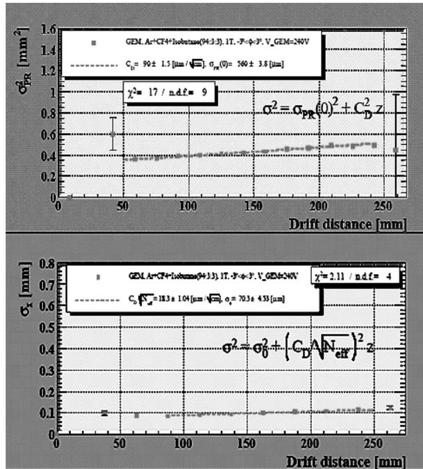
Fig.2 The width of the pad response (top) and the spatial resolution (bottom) as functions of the drift length. The gas is Ar(94%)-CF<sub>4</sub>(3%)-Isobutene(3%) gas mixture. The dotted line in each plot is the best fit to the data by the function given in the plot.
