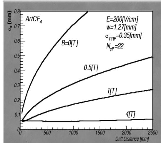
Fig.1 The R $\phi$  spatial resolution of GEM TPC calculated by the analytic formula for Ar(97%)-CF<sub>4</sub>(3%) gas mixture in the magnetic field up to 4T [3].
