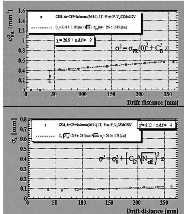
Fig.3 The width of the pad response (top) and the space resolution (bottom) as functions of the drift length. The gas is Ar(96%)-CF<sub>4</sub>(3%)-iC<sub>4</sub>H<sub>10</sub>(1%) gas mixture. The dotted line in each plot is the best fit to the data by the function given in the plot.
