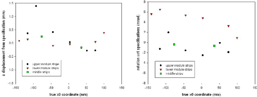
**Figure 4.** On the left is shown the difference between the specified and measured horizontal coordinates for the aluminum strips at the centre line of the TPC. The right figure shows the difference between the specified and measured azimuthal angles of the strips.
