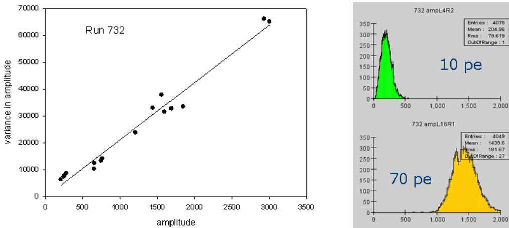
**Figure 3.** On the left is shown the observed relation between variance and amplitude for different sets of pads from laser events. This appears to be linear as expected for a Poisson process, thereby allowing for a direct estimate of the absolute gain of the system. On the right are shown the distribution of amplitudes for two selected pad groups and the estimated mean number of photoelectrons responsible for the signals.
