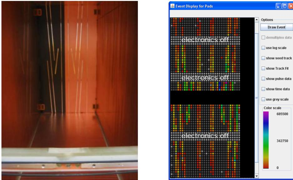
**Figure 2.** The photograph on the left shows a view inside the T2K prototype TPC built in Canada in 2005. The central cathode surface on the left is carbon loaded kapton, and copper on the right. The aluminum strips are clearly visible. On the right is an event display, showing the amplitude of the signals on the readout pads after a single flash of the UV laser.
