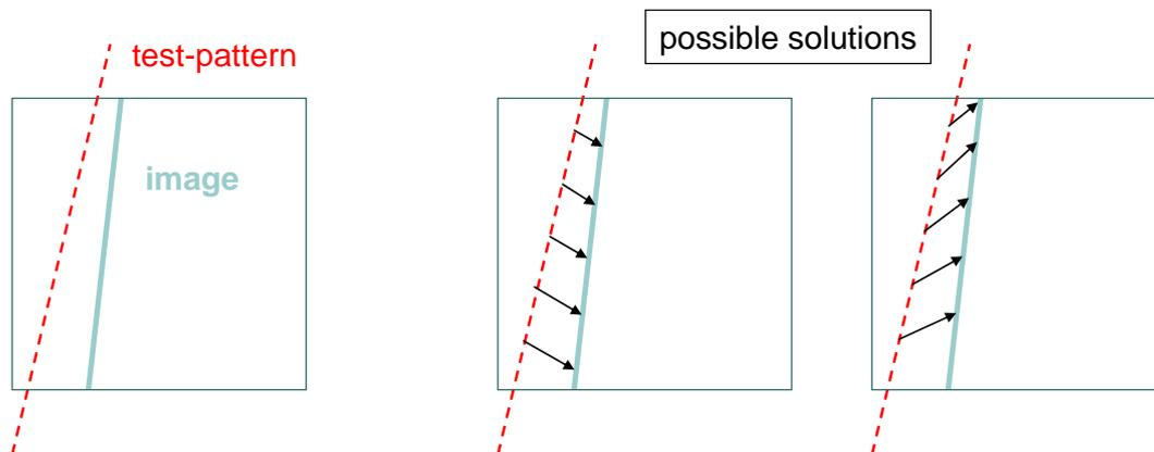
**Figure 1.** The left figure shows the test pattern projected onto the endplate and an observed image in the case of a large distortion in the drift lines of the electrons. On the right are shown two possible solutions that can produce the observed effect to illustrate the ambiguity that arises when using strips as test patterns.
