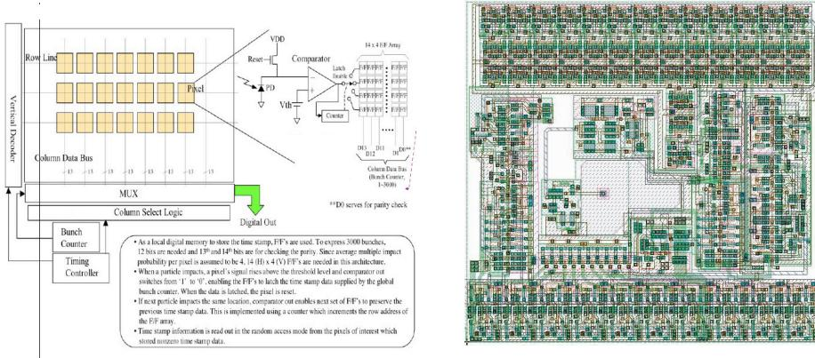
Figure 2: Chronopixel Array Architecture
