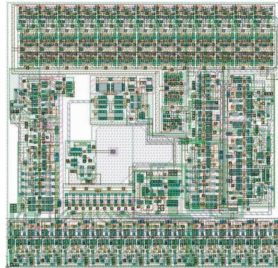
Figure 3: Image of the 645 transistor pixel design
