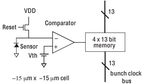
Figure 1: Pixel Architecture
