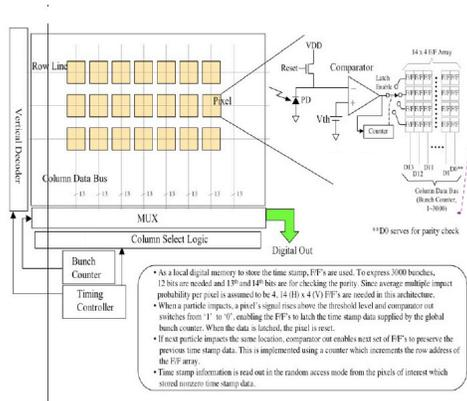
Figure 2: Chronopixel Array Architecture
