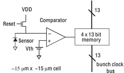
Figure 1: Pixel Architecture
