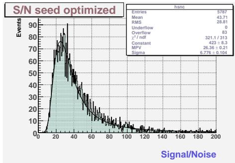
Figure 1: SNR measured at the CERN-SPS with MIMOSA-9, ( $20 \mu\text{m}$  pitch) at  $T = 20^\circ\text{C}$ .
