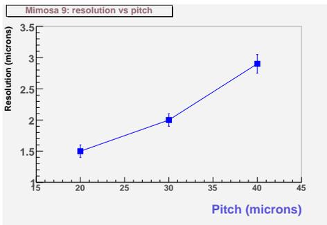
Figure 2: Single point resolution measured at the CERN-SPS with MIMOSA-9 (three pitch values: 20, 30 and  $40 \mu\text{m}$ )
