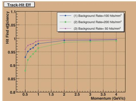
Figure 2: Efficiencies on Layer 2 under the background levels at 50, 100 and 200 hits/mm<sup>2</sup>/train.
