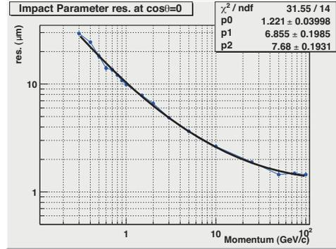
Figure 1: The momentum dependence of the impact parameter resolution.
