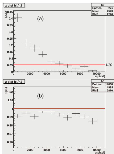
Figure 3: Z-dependent of Rejection factor for the pair background (a), and 1 GeV/c muon tracks (b), where unit of horizontal axis is a pixel.
