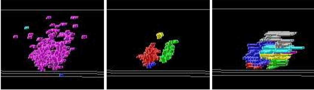
Figure 1: Display of a single 10 GeV  $\pi^0$  event. Left: standard GLD clustering with  $1 \times 1$  cm cell size; Centre: “track” clustering with  $1 \times 1$  cm cell size; Right: “track” clustering with  $5 \times 1$  cm cell size. Different colours denote separate “tracks”.
