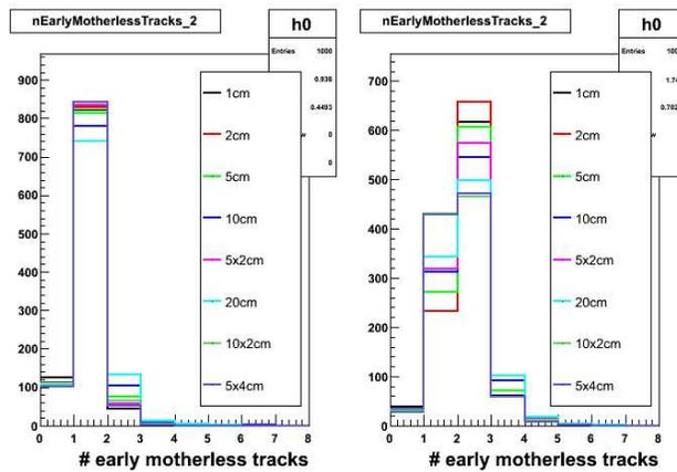
Figure 2: Number of early mother-less tracks reconstructed in 10 GeV photon (left) and  $\pi^0$  (right) events. Different color histograms are the results of different strip shapes and sizes.
