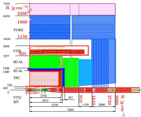
Figure 1: Quadrant of a typical ILC detector [4], length units in mm; amount of material indicated by  $R [\text{g cm}^{-2}]$
