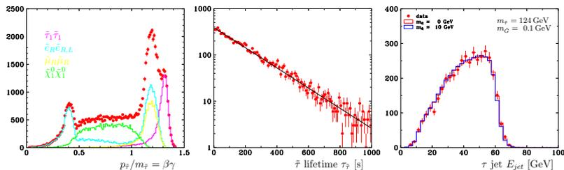
Figure 3: SPS 7 scenario, assuming  $\mathcal{L} = 100 \text{ fb}^{-1}$  at  $\sqrt{s} = 410 \text{ GeV}$ : (a)  $\tilde{\tau}$  production spectra of scaled momentum  $p/m = \beta\gamma$  with contributions from various processes; (b)  $\tilde{\tau}$  lifetime distribution; (c)  $\tau$  jet energy spectrum of the decay  $\tilde{\tau}_1 \rightarrow \tau\tilde{G}$  compared with simulations of  $m_{\tilde{G}} = 0 \text{ GeV}$  and  $10 \text{ GeV}$
