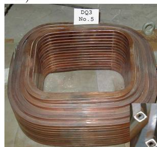
Figure 3: Dipole coil made from conductor with mineral insulation
