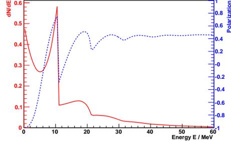
Figure 2: Energy (red) and polarisation (blue) of photons created in a helical undulator.
