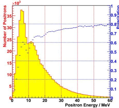
Figure 3: Energy (red) and polarisation (blue) of positrons after the production target of thickness  $d = 0.4X_0$ .
