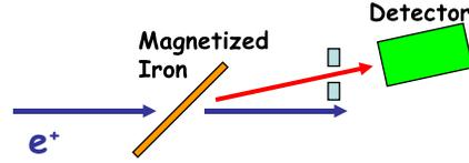
**Figure 2:** Sketch of a Bhabha polarimeter. Behind the target an appropriate mask system selects the angular range of interest.
