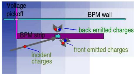
Figure 4: Hits and emission from BPM striplines.
