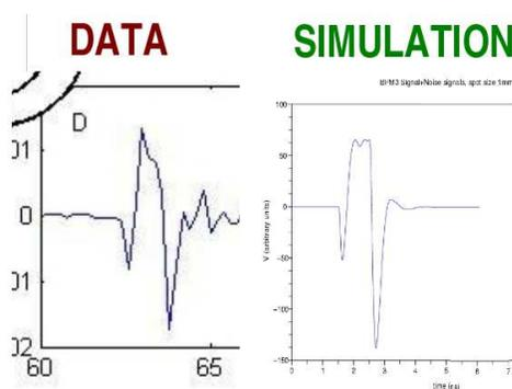
Figure 6: high spray mode BPM voltage signals.
