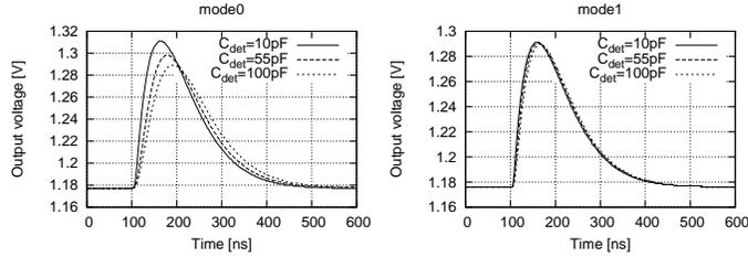
Figure 3: Example of shaper output in calibration mode for 10fC input charge (mode0) and in physics mode for 1pC input charge (mode1)
