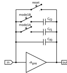
Figure 4: Schematic of switched-reset preamplifier
