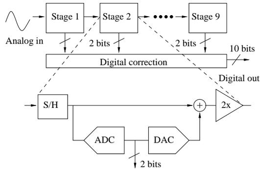
Figure 5: Pipeline ADC architecture
