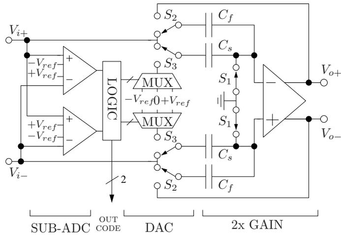
Figure 6: Simplified schematic of a 1.5 bit stage. Switches set to  $\varphi_1$  phase
