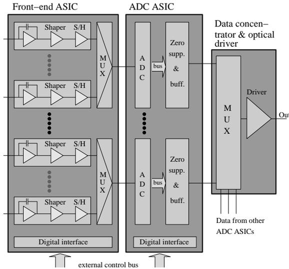
Figure 1: Block diagram of the LumiCal readout electronics
