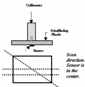
**Figure 1: Scan apparatus**
