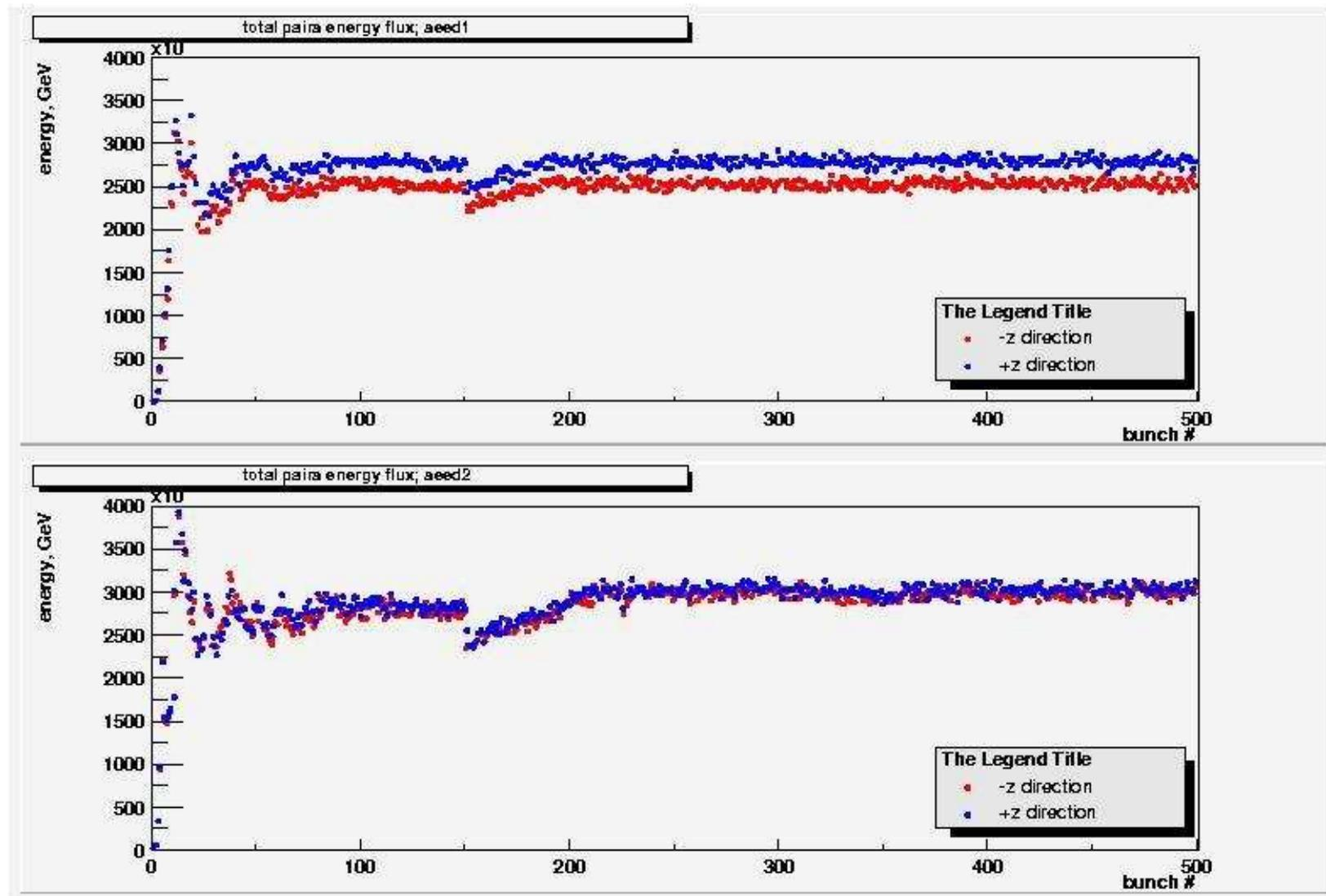
Difference between directions due to the beam-beam interaction on different bunch shapes
