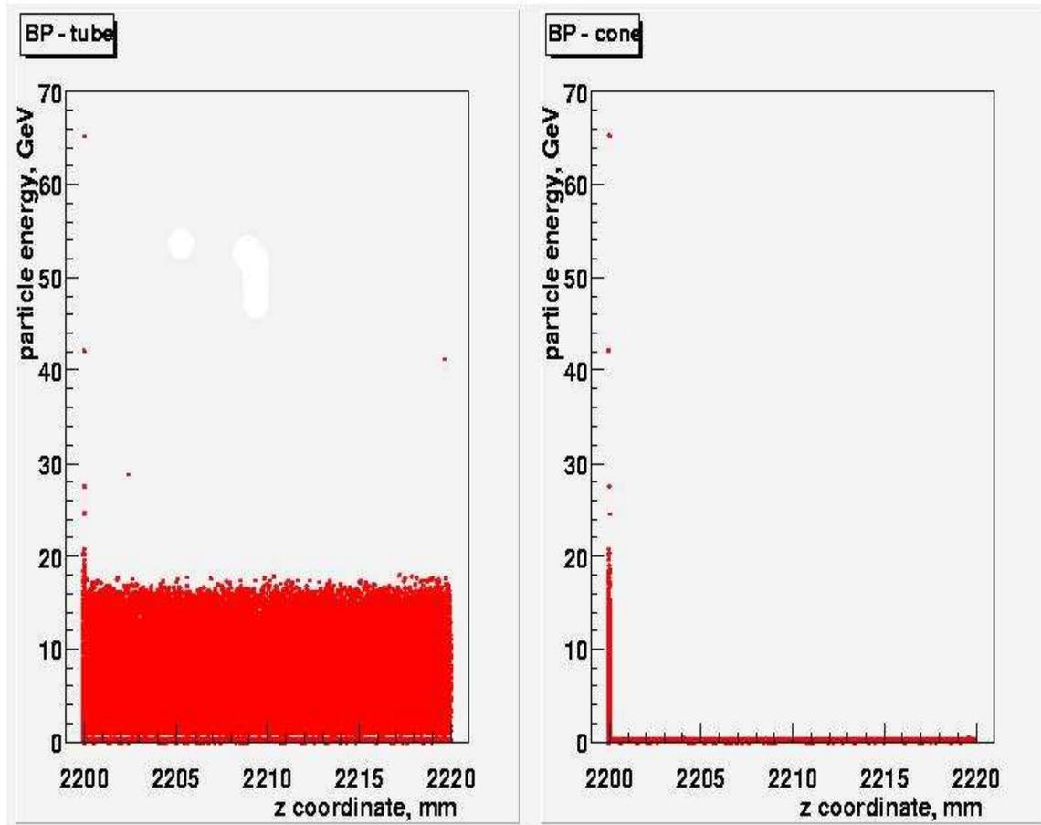
Each point on the plot corresponds to  $e^+$  or  $e^-$  with energy  $E$  hitting BP from inside at  $z$  coordinate
