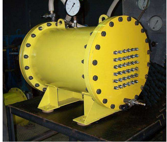
Fig. 11. A picture of the heavy gas ionization chamber used for testbeam studies at the PS of the IHEP Protvino.
