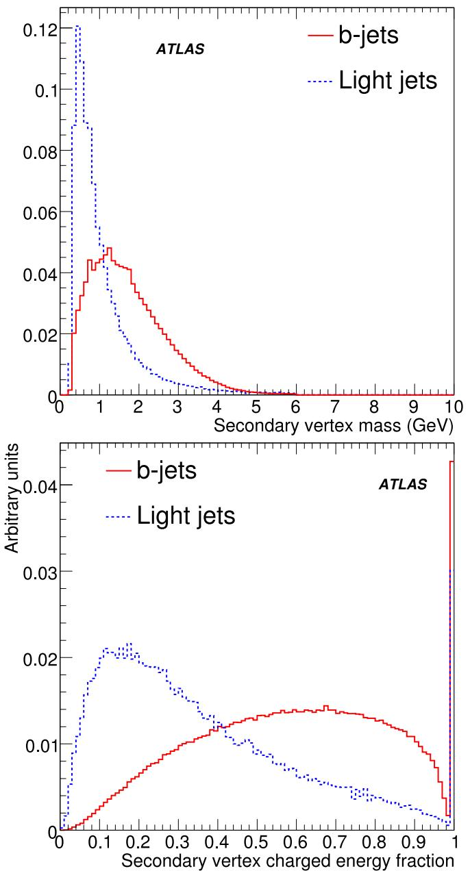
With the available methods e.g. a light quark rejection of  $10^3$  and a c-quark rejection of 10 can be achieved for 50% b-efficiency ( $t\bar{t}$  events)
