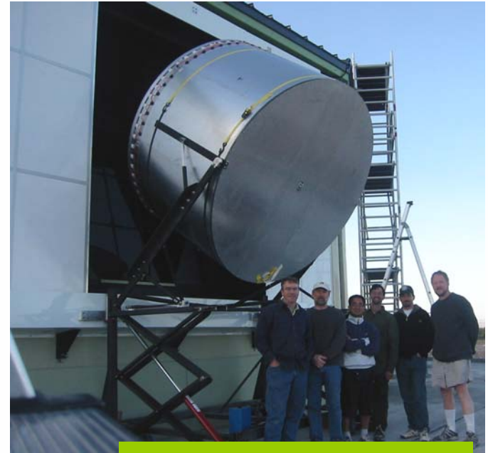
Drum for uniform camera illumination: end to end calibration
