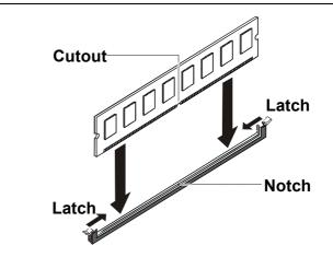
Install the DIMM module into the socket (A) and press it firmly in until it seats correctly (B):
