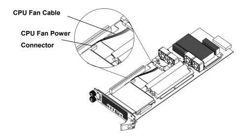
Figure 11: Removing CPU Fan Cable
