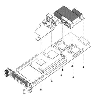
Figure 12 : Removing CPU Fan/Heat-sink
