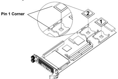
Figure 13: Installing CPU
