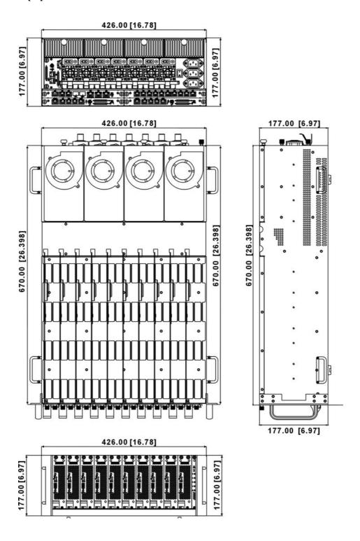
Figure 17: HS420 series chassis dimension
