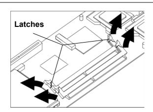
2. Align the memory module with the socket. The DIMM sockets are keyed with notches and the DIMMs are keyed with cutouts so that they can only be installed correctly. Check that the cutouts on the DIMM module edge connector match the notches in the DIMM socket.
