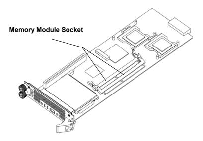
Figure 15: Memory module socket location
