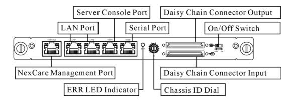
Figure 7: Basic Management Blade and Advanced Management Blade
