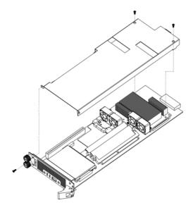
Figure 10 : Open the server blade cover
