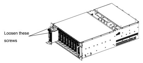
Figure 9: Remove server blade from the chassis
