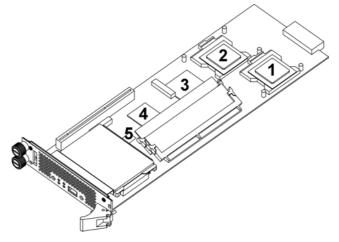
Figure 14: Location for applying thermal compound
