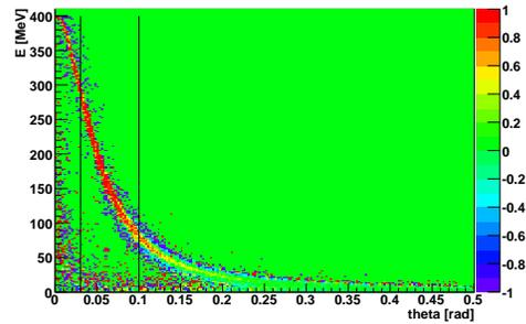
**Figure 4:** Asymmetry of the  $E - \vartheta$  distribution of the Bhabha electrons. The vertical lines indicate the angular range of highest asymmetry.
