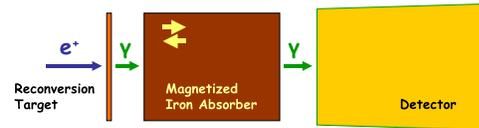
**Figure 5:** The principle of a Compton transmission polarimeter
