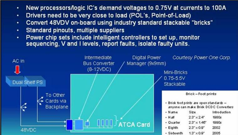
Figure 3: Board Level Intelligent Power System
