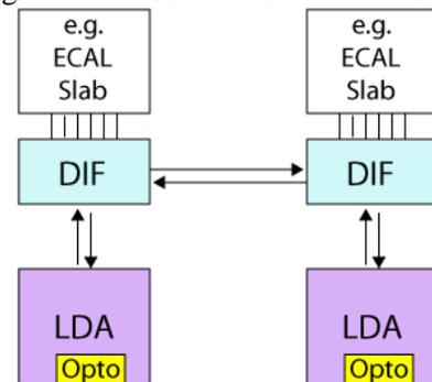
**Figure 3: Schematic of the DAQ links between the front end electronics and first level concentrator (LDA).**
