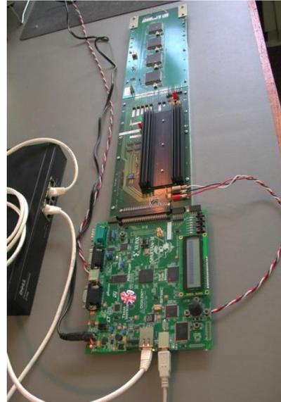
**Figure 2: Prototype DIF connected to simulated EUDET ECAL VFE electronics.**
