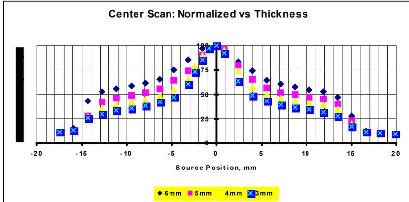
Figure 2: Scan measurements through the center for different thicknesses.
